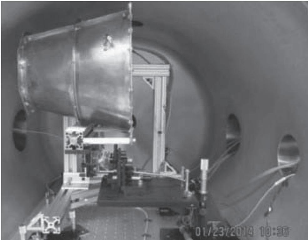
**Fig. 4 EM drive on balance, inside vacuum chamber [8]. Large diameter of the EM drive (also called RF cavity in vacuum) is 27.94 cm, small diameter is 15.88 cm and the length is 22.86 cm.**
